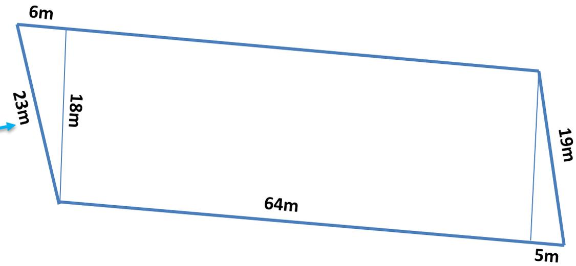
面積計算:  $\{(64 \times 18) + (6 \times 18 / 2) + (5 \times 18 / 2)\} = 1251 \text{m}^2$
